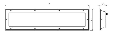
M600 SQ 595 x 595 x 87 mm M598 SQ 598 x 598 x 87 mm M623 SQ 623 x 623 x 87 mm **M625/PB** SQ 620 x 620 x 87 mm R 1195 x 295 x 87 mm R 1198 x 298 x 87 mm R 1247 x 312 x 87 mm R 1245 x 310 x 87 mm
