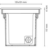
HOLE FOR RECESSING 123x123 mm
