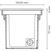
HOLE FOR RECESSING 123x123 mm
